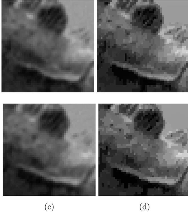
Figure 12: Close-ups of images captured in the presence of (1st row) translation and (2nd row) rotation, (c) by the previous method of multi-exposure [14], and (d) by the proposed method of multi-exposure.
